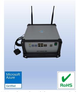
The ECT-MAN computer is used in the Ectron SmartEYE<sup>TM</sup> platform. ECT-MAN can be used stand alone as a standard gateway, control computer, server class edge computer, mobile server and comes preloaded with edge AI/ML capability. Suitable for use as a in conjunction with multiple Ectron Edge computers as an aggregator or stand alone with Hub where sensors are aggregated. Like all Ectron Edge computers can bridge OT-IT protocols
