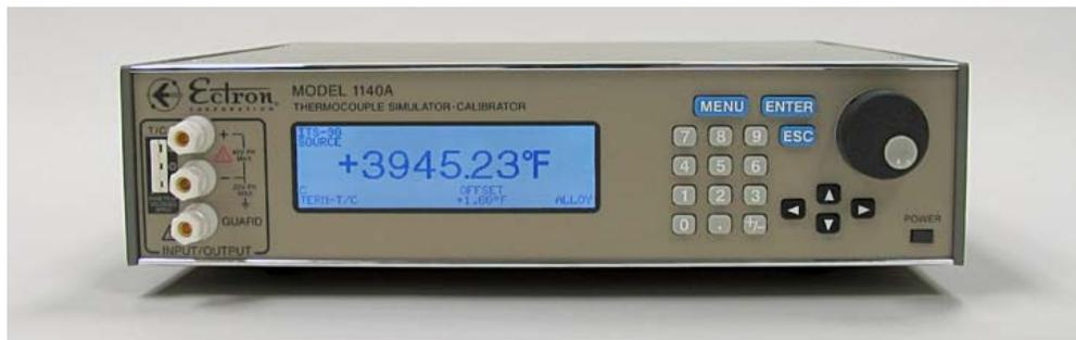
The **Model 1140A** provides four calibration functions: precise simulation of thermocouple signals, precise measurement of thermocouple signals, generation of accurate dc voltages from microvolt level to  $\pm 11$  V dc, and measurement of dc voltages over the same range. The thermocouple simulation and measurement accuracies are the highest in the industry, affording a margin of calibration accuracy heretofore unavailable.
