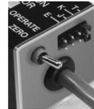
Jumper block at right selects type E, J, K, or T thermocouple. The toggle switch at left can be switched to the ZERO position to provide a shorted output for amplifier zero adjustment.
